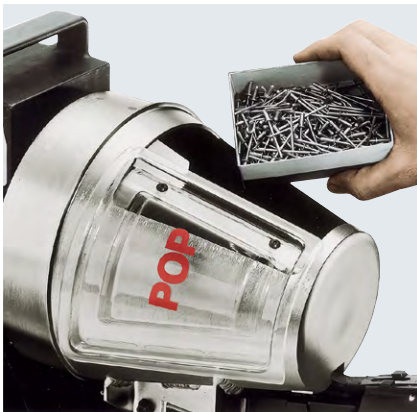
Fill the container with approx. 1000 blind rivets (see filling mark)
